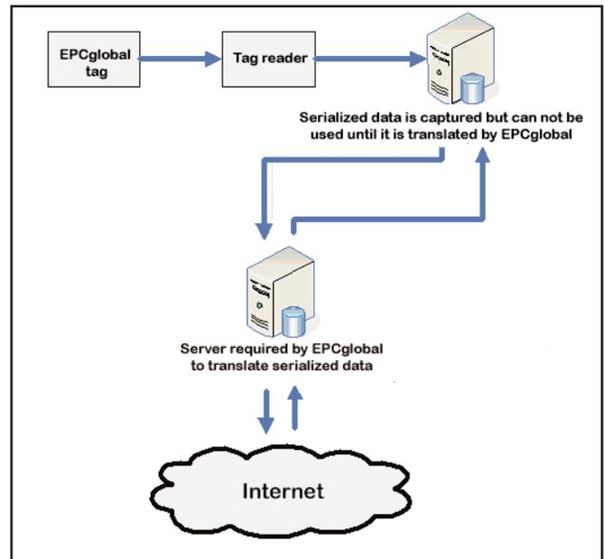
The EPCglobal approach requires numerous steps to access information. Because the EPCglobal tag contains a coded serial number, it must be cross-referenced to yield the required data.
