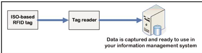
The ISO approach is based on simplicity and direct access to information. The ISO tag is self-contained with all required information.
