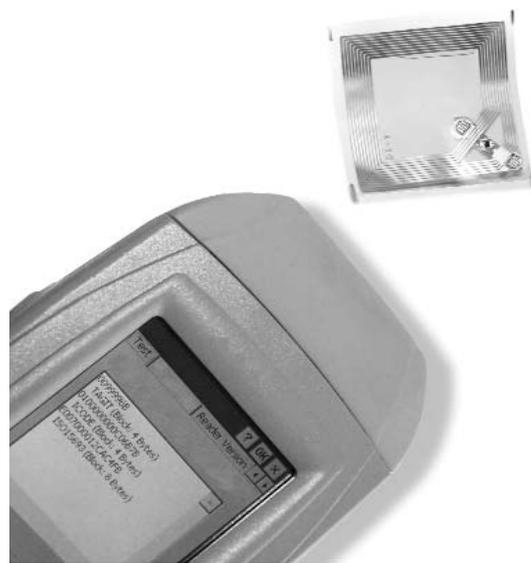
Figure 2 - RFID tag communicates with a mobile reader
